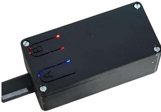
Fig. 1 Prototype of the GaSens device for monitoring of environmental parameters.
