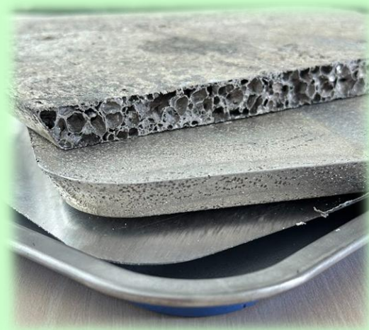
Thermal battery panel PCM RT44HC (dT±20°C)
