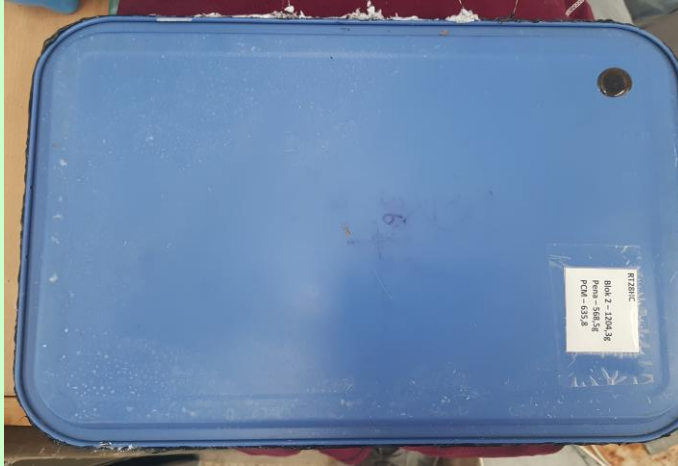
Thermal battery panel PCM RT44HC (dT±20°C)
