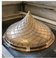
VACUUM FORMING OVER MOLD
