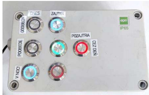
Fig. 2: Demand-side UI device for selecting the operational window while running appliances
